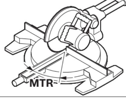
Press button **15** again. “**MTR**” and the calculated miter angle for the chop and miter saw are indicated on the display.
