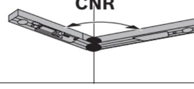
To measure the corner angle, place the fold-out and base legs flat against the walls and read the measured corner angle or set a known corner angle on the anglefinder.
