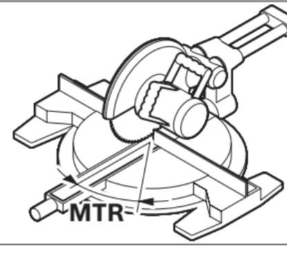
Press button **14**. The calculated horizontal miter angle “**MTR**”, which has to be set on the chop and miter saw, and the “**MTR**” indicator will be shown on the display.
