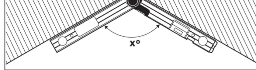
When workpieces are to be fitted into a corner (e.g. for floor trimmings), measure the corner angle **x°** by applying the fold-out leg and the base leg. For given angles (e.g. picture frames), open the fold-out leg and the base leg until the desired angle is indicated in the display.
