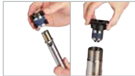
1) Insert pre-oiled packing cartridge assembly
